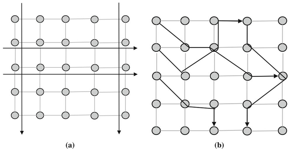
Fig. 15 Aggregate throughput in grid topology: (a) Aggregate throughput for aligned traffic flows in grid topology and (b) Aggregate throughput for random unaligned traffic flows in grid topology
