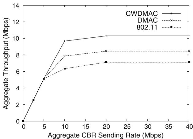
**Fig. 16** Aggregate throughput in a 30 node random topology
